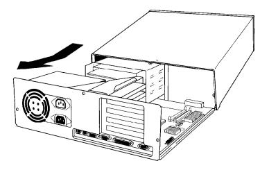
2. Lower the cover and slide it straight back over the computer until it cannot go any farther.
